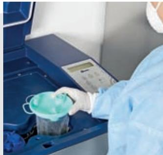
Steelco FLY CUTTER drainage bag thermidisinfector as a cutting device is designed to guarantee the nursing staff to be absolutely physical secure. Drainage bags simply have to be inserted in the special support inside the machine with no contact with other parts except cover and control panel. The machine is equipped with all needed safety devices.
